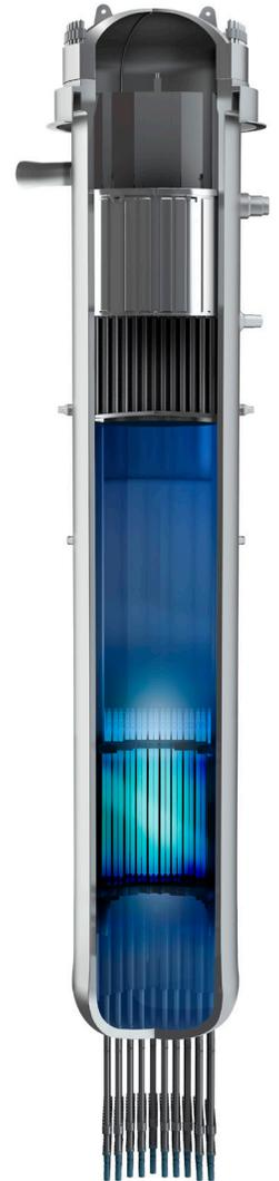
\*Economic Simplified Boiling Water Reactor - 1520 MWe Generation III+ boiling water reactor
