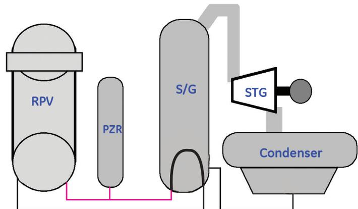
The water in the reactor is pressurized so it does not boil. This heated water then passes through a heat exchanger called a steam generator. The heat from the steam then converts another loop of water to steam, which drives the turbine to produce power.
