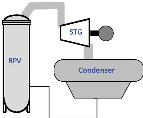
The reactor heats the water and turns it directly into steam. The steam drives a steam turbine, which spins a generator to produce power.
