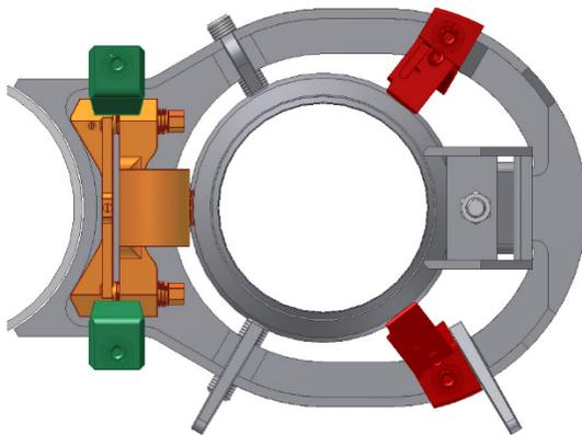
For Aging BWR Plants the GEH Jet Pump Anti-Vibration System (AVS) is the Solution for Mitigating damage due to Flow Induced Vibration among Jet Pump Repairs because of its ability to restore and assure continued positive three-point contact. The GEH AVS provides customers: “Wear due to Jet Pump Vibrations will be reduced, which will increase safety, reliability, and outage efficiency”.
